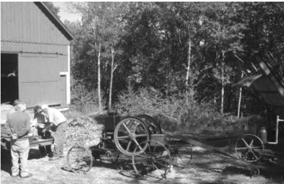
An Attraction Provided by Bill Roberts (white shirt at left) at the Annual Picnic Was a 6 hp 100 yr old Abenague Engine (right), Running an Antique Water Pump Using a Belt Drive. This Engine is the Same Model as Used by Rod and Fred Doolittle's Father on the Doolittle Farm Which Sat at the Bottom of the Hill Below the Visitor Center.
